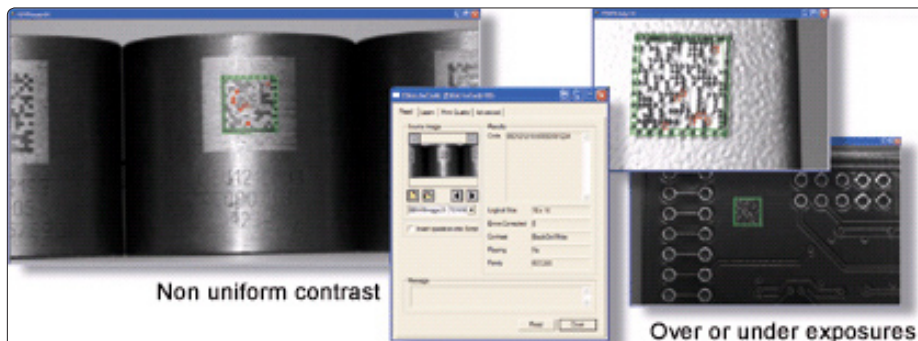
Camera Based Automatic 2D MatrixCode Reader Software supporting Multiple Readers on one PC.
